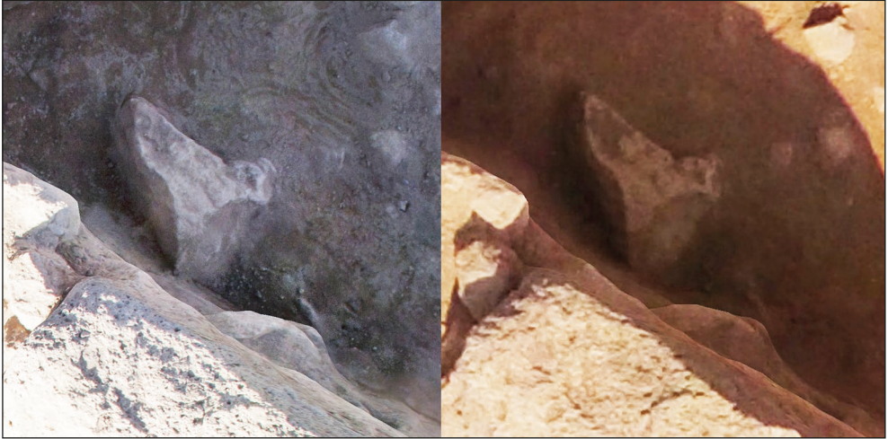
Fig. 3. Two magnified fragments of orthophotos covering the same area: left, created from close-range images taken early in the morning and right, generated from photos taken in the afternoon at higher altitude with an UAV. Note the difference in sharpness and visibility (Photos M. Truszkowski, O. Bagi)
