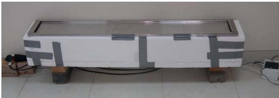
Fig. 4. Custom-built container for the alkaline sulphite bath in use at the site (PCMA UW PMSaruq Project, Dubai Municipality/photo W. Weker)
