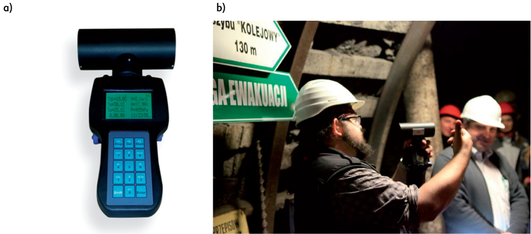
Figure 4. Apparatus at the station for testing the air flow rate using ultrasonic waves:
