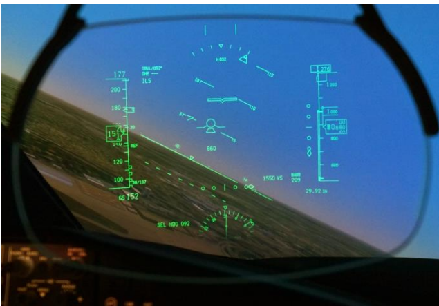
Fig. 6. Composite information displayed by HUD in aeroplane
