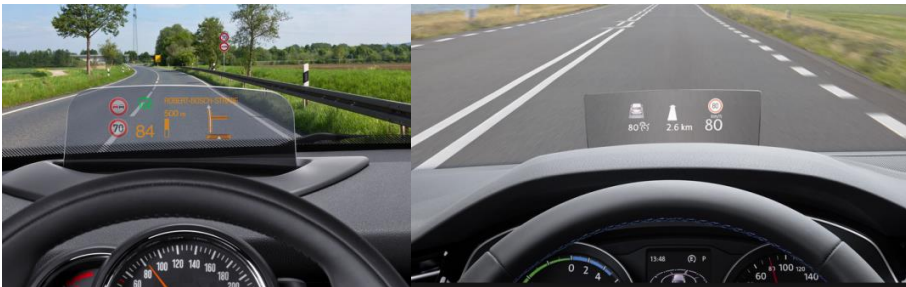
Fig. 10. Example of HUD with data projection on optical combination plate in automobile
