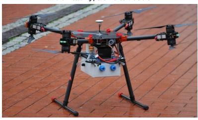
Picture 3. Measuring platform under the drone
