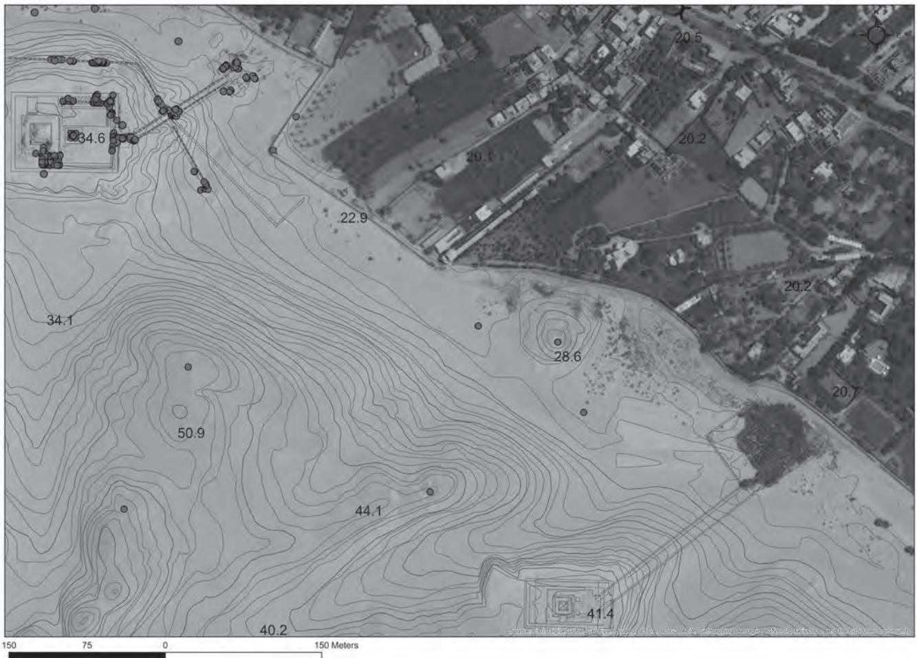
Fig. 15 The 2017 topographical survey of the Abu Ghurab area overlaid with a Google Earth image and the French-Egyptian 1978 photogrammetric map (EMHR 1978, sheet 21, scale 1:5000; elaboration by E. Brienza)
