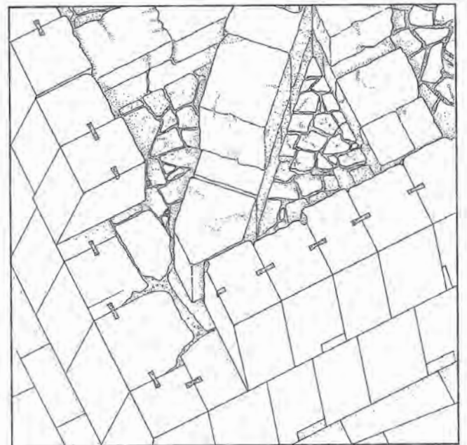
Fig. 4b Scheme of the building technique of the core masonry of the “pedestal building” (adapted after Arnold 1991: fig. 4.109). Differently from Arnold’s scheme, which refers to the pyramid of Sesostris I, the blocks of the “pedestal building” are not adjoining one another by means of dovetail cramps but simply juxtaposed
