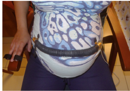
Fig. 3. Pneumograph on the abdomen (Lafayette).
