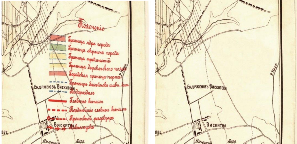
Fig. 3. A fragment of a map of the City of Lodz and surrounding areas on a scale of 1:25 000 from 1909 transformed using spline transformation before and after correction involving the removal of the legend
