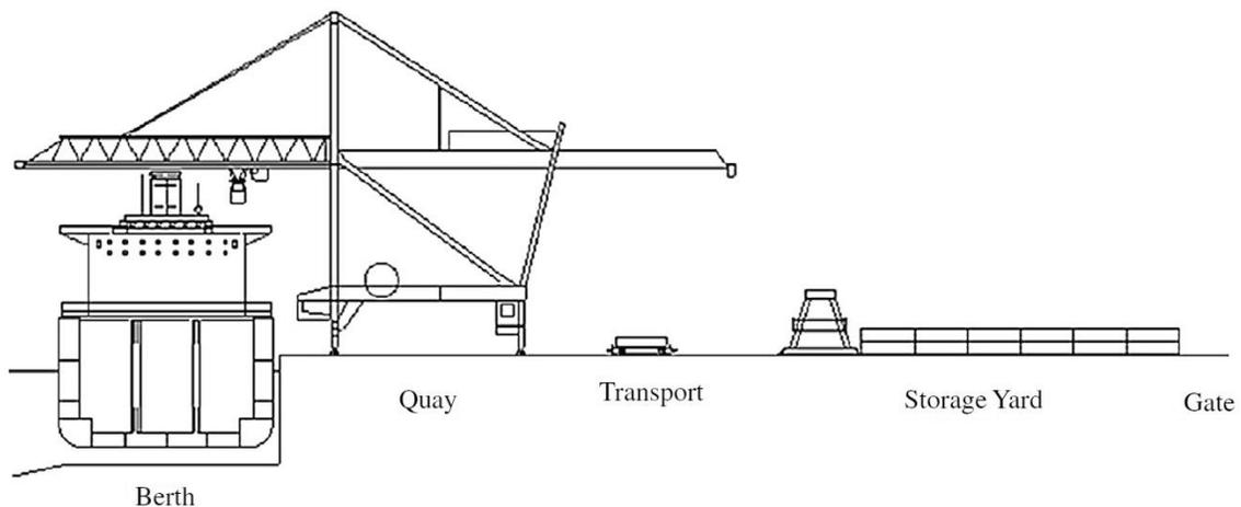
Fig. 2. A conceptual diagram of the containers terminal with its main areas [1].
