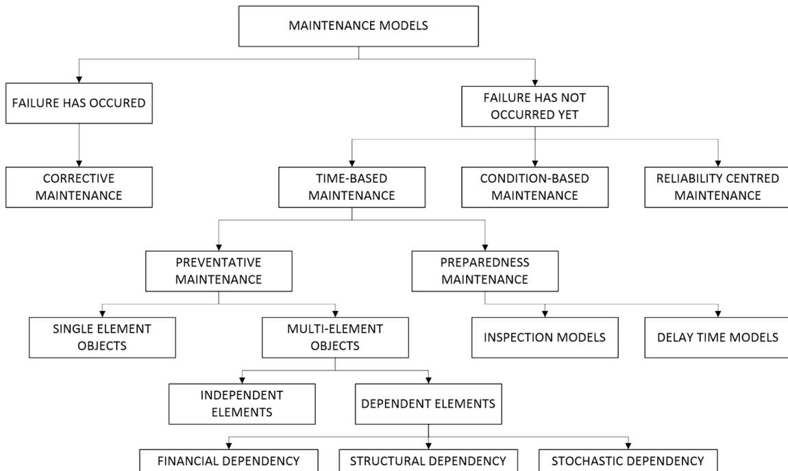
Fig. 4. Classification of principal models of a technical object maintenance, based on [15].
