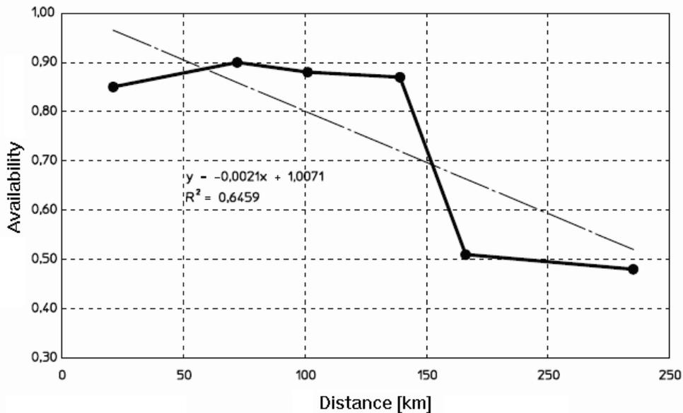
Fig. 6. Dependence between availability and the distance between the place of operation and the place of production. Reproduced from: [17].
