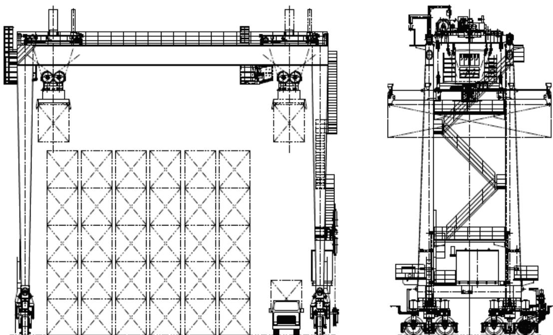
Fig. 5. A typical RTG crane – HDHM reference materials [9].
