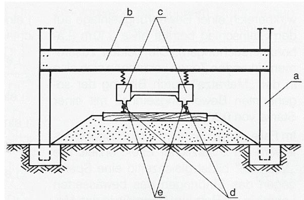
Fig. 1. Traverse section of the test bench, done in CNTK [Mazur, Surowiecki 1989; Surowiecki 2011]: a - pillars of framework structure, b - crossbar, c - cylinder generating vertical load on the rails, d - rail, e - the ends of cylinders transmitting the load onto the rails
