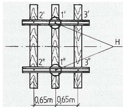
Fig. 2. The plan of track section model, consisting of three sleepers [Mazur, Surowiecki 1989, Surowiecki 2011]: H - hydraulic cylinder pressure points which generate the vertical load on rails
