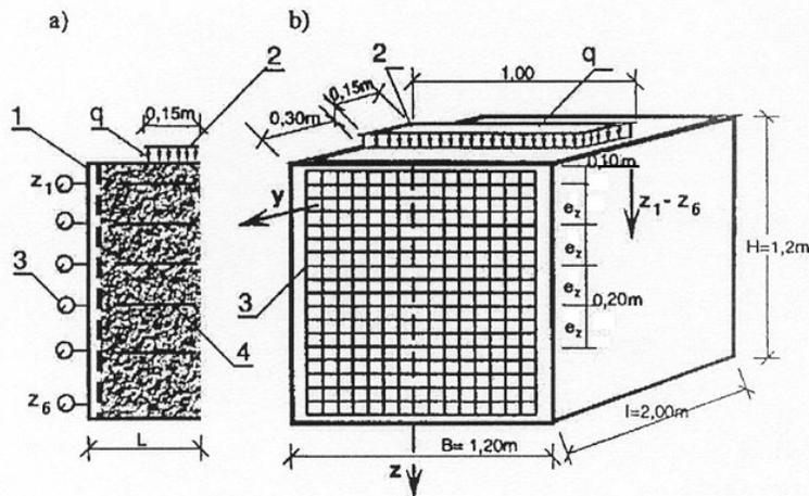
Fig. 4. The scheme of the test bench [Surowiecki 2004, 2011]: *a* - vertical cross section; *b* - general view; 1 - retaining wall (measurement) model, 2 - loading plate 0.15 x 1.0 m, 3 - horizontal displacements sensors; 4 - reinforcement inserts;  $z_1$ - $z_6$  - measuring levels
