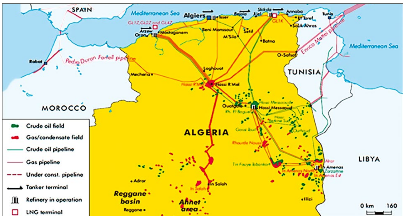
Figure 2. Energy infrastructure in Algeria
