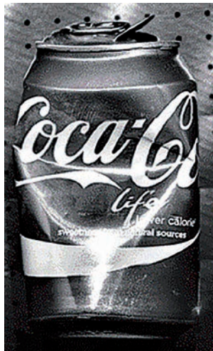
Fig. 18, 19. A can with fingerprints revealed with Magnetic Fluor Red powder.
