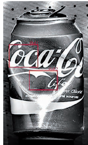
Fig. 18, 19. A can with fingerprints revealed with Magnetic Fluor Red powder.
