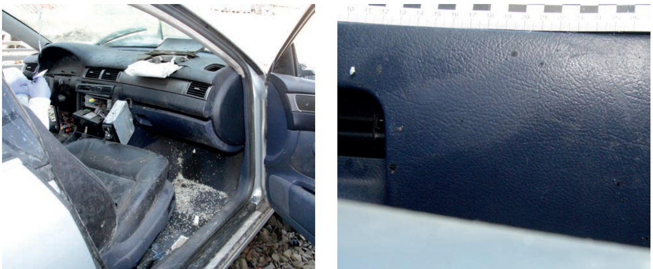
Fig. 8. Interior of the AUDI A6 vehicle tested and a close-up of the scratches found on the surface of the glove compartment door.
