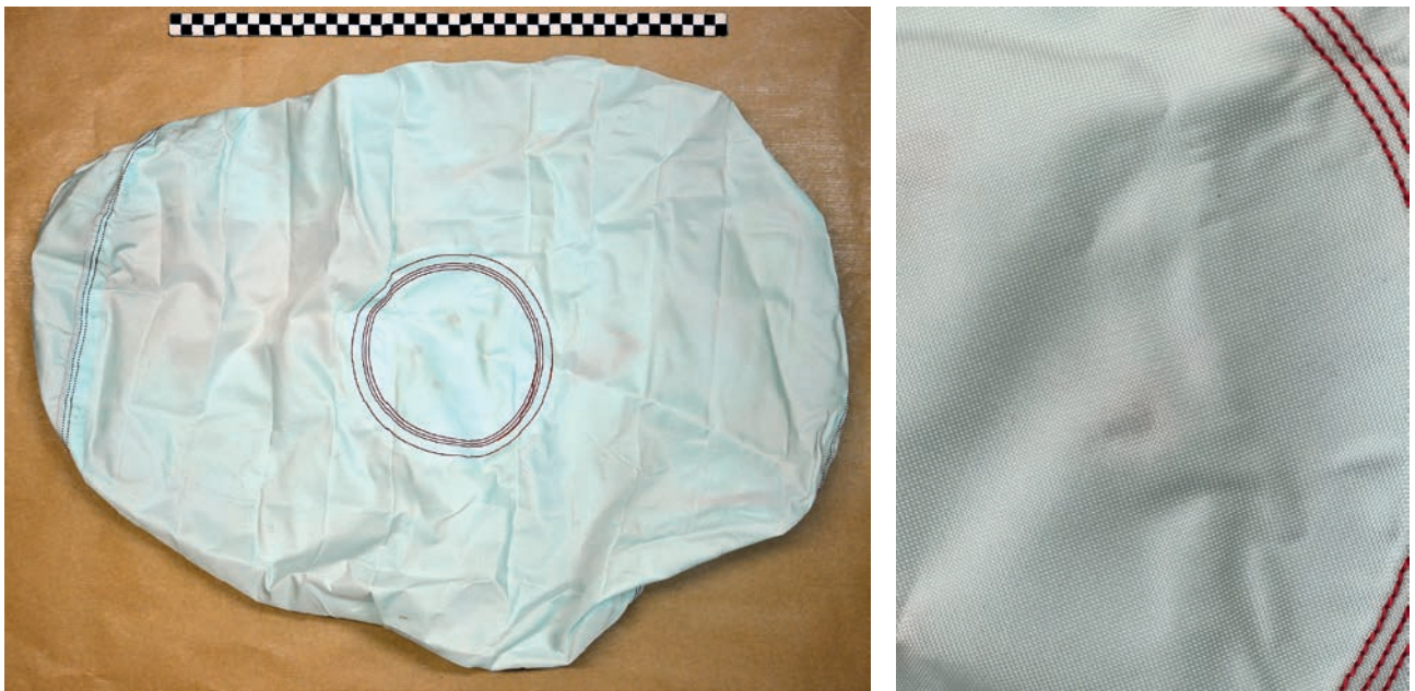
Fig. 4. Deployed driver airbag and close-up of a fragment of this airbag containing a delicate print that looks like a print of some textile
