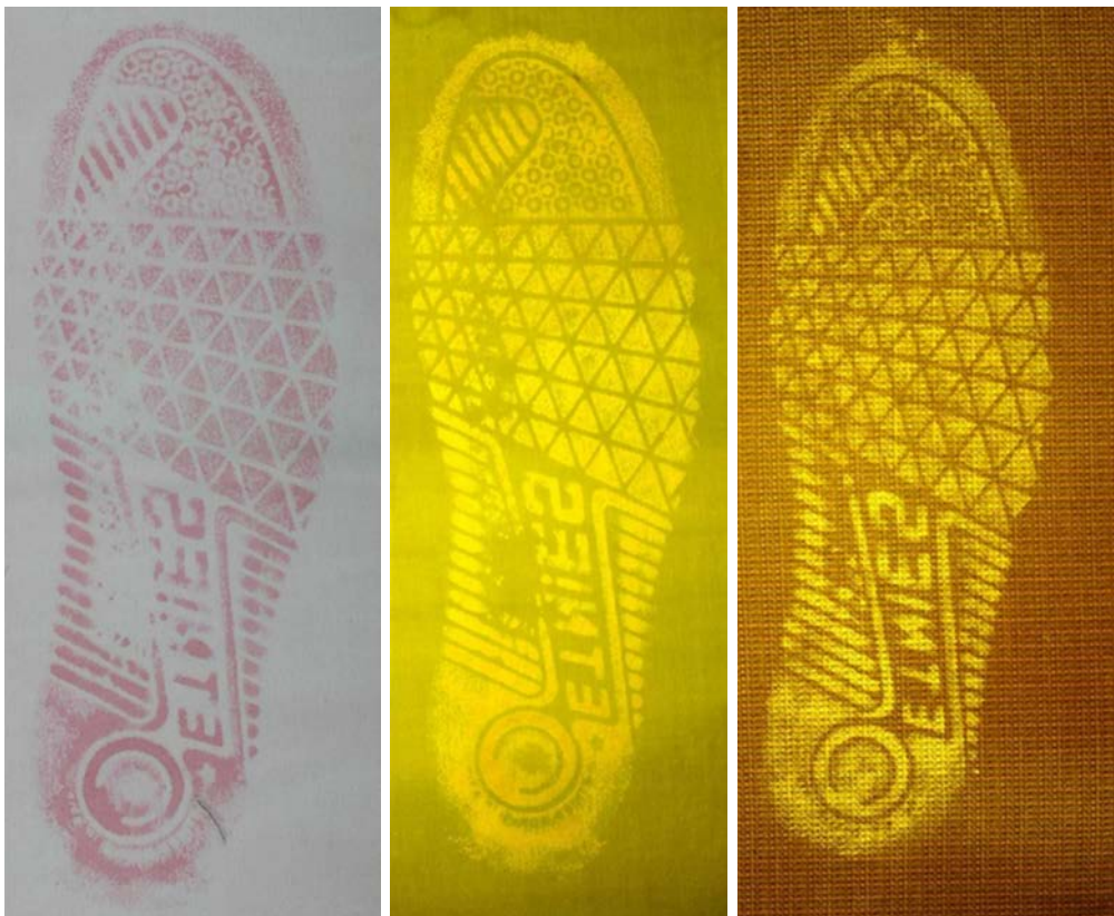
Fig. 44, 45, 46. Urine footwear impressions on cotton surfaces visualised by DFO, visible in white light (left) and in fluorescence (middle and right)
