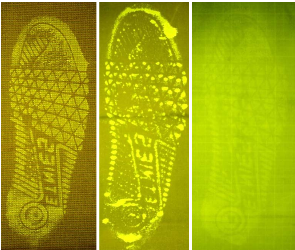
Fig. 47, 48, 49. Examples of footwear impressions left by urine on textile surfaces, visualised by DMAC
