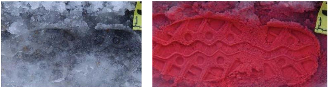
Fig. 10, 11. Three-dimensional snow impression before (left) and after (right) contrasting with Snow Print Wax
