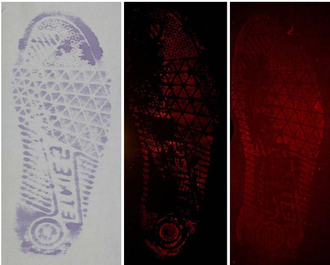
Fig. 26, 27, 28. Blood footwear impressions visualised by LCV visible in white light (left), in fluorescence (middle), and in fluorescence when the light source is laser (right)
