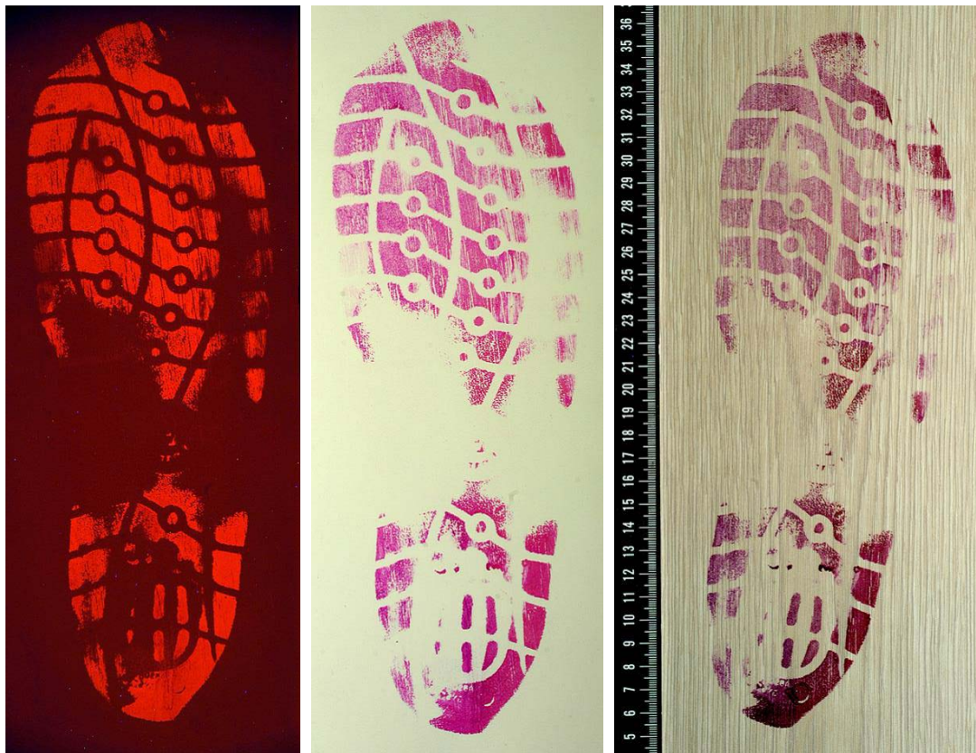
Fig. 17, 18, 19. Blood footwear impressions visualised by Hungarian Red visible in white light on the surface (left) and after being transferred from the surface to a white gelatin lifter visible in white light (middle) and fluorescence (right)
