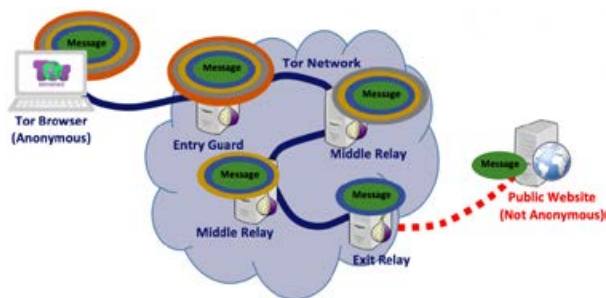
Fig. 3. A diagram showing how a message travels through the Tor network until it reaches a public website. The Tor network client (Tor Browser) adds as many layers as there are relays in the chain
