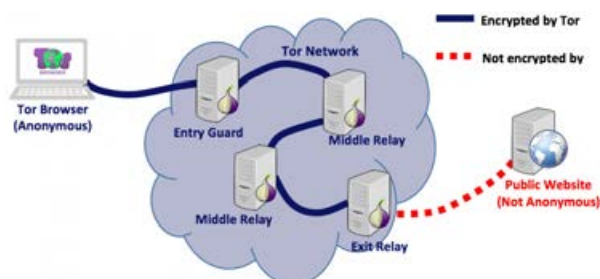
Fig. 2. Diagram showing a typical scenario of a Tor client accessing a public site on the Internet
