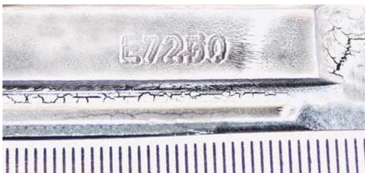
Fig. 9. The number was revealed using a defectoscope
