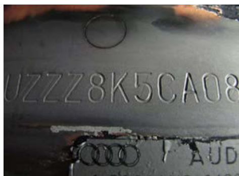
Fig. 6. Destructive testing using the recrystallisation phenomenon
