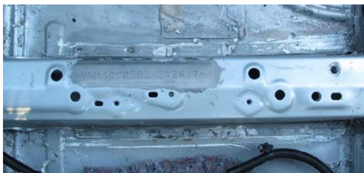
Fig. 7. Destructive testing – removal of paint to assess the connections of the element containing the VIN number to the rest of the bodywork
