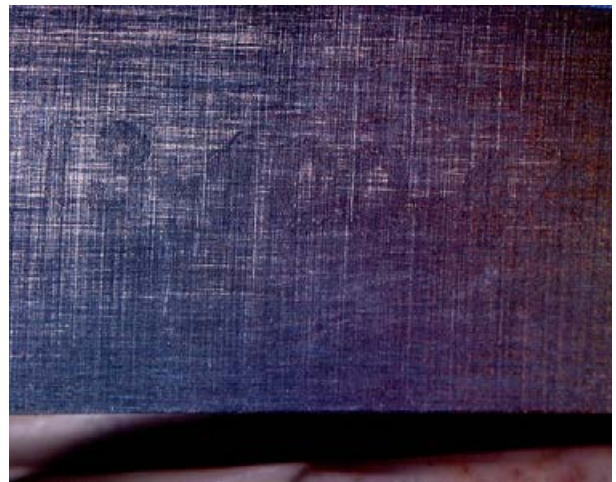
Fig. 13. Marking of surgical instrument numbers reproduced with chemical reagent
