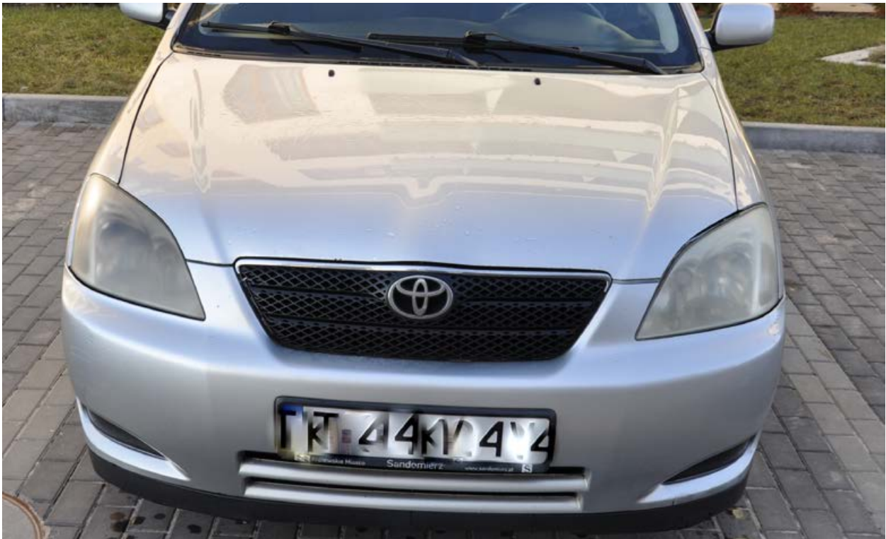
Fig. 1. Research vehicle with dulled headlights installed
