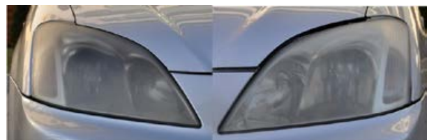
Fig. 6. Headlights in service (dulled)
