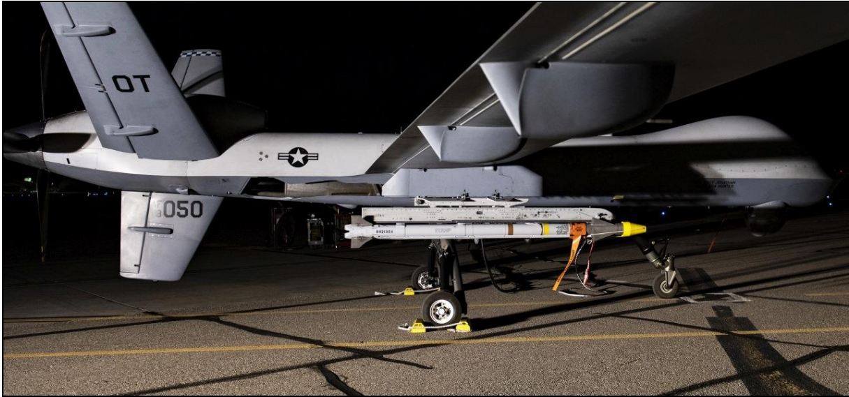
Figure 2. MQ-9 armed with the AIM-9X Block 2 missile. Adopted from: “MQ-9 Reaper new weapons test”, US Air Force, by A.H. Stevens, Copyright 2021 by the Publisher https://www.konflikty.pl/wp-content/uploads/2021/02/200903-F-UA265-1057.jpg
