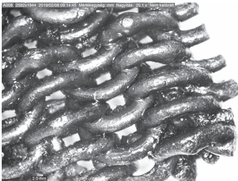
Fig. 7. On the microscope photo of the Csengersima mail, thickening of the rings referring to welding can be well observed
