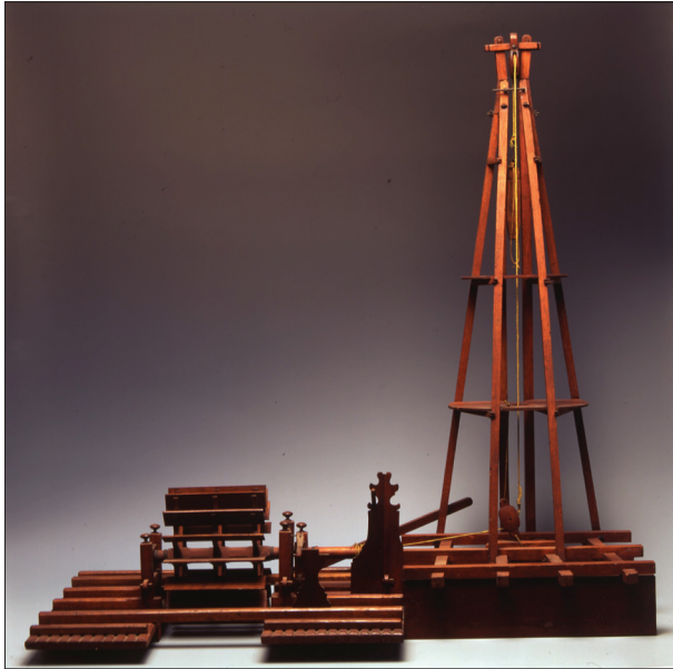
Fig. VII. Model of the pile-driver designed and made by Bartolomeo Ferracina for the reconstruction of the bridge designed by Palladio in Bassano, Cabinet of Physics of Giovanni Poleni. Museum of the History of Physics, University of Padua. Photo F. Zannini
