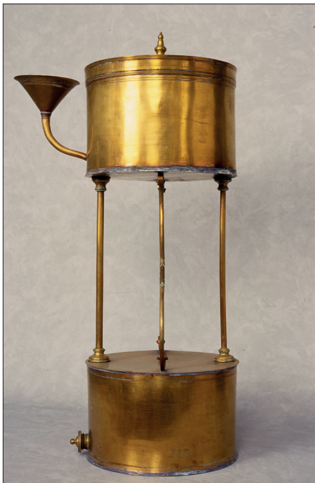
Fig. II. Hero's fountain, mid-eighteenth century, Cabinet of Physics of Giovanni Poleni. Museum of the History of Physics, University of Padua. Photo F. Zannini
