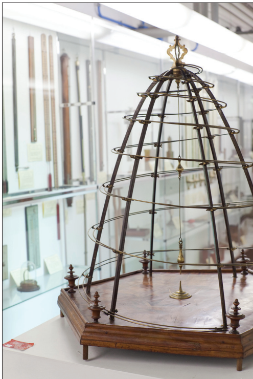
Fig. VIII. Instrument designed to demonstrate Galileo's law of falling bodies, made by Philippe Vayringe, Cabinet of Physics of Giovanni Poleni. Museum of the History of Physics, University of Padua. Photo M. Pistore
