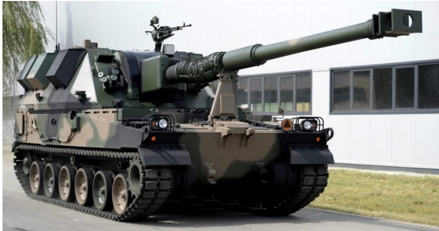
Fig. 1. 155 mm self-propelled howitzer 'Krab' on the South Korean K9 'Thunder' chassis by Samsung Techwin
