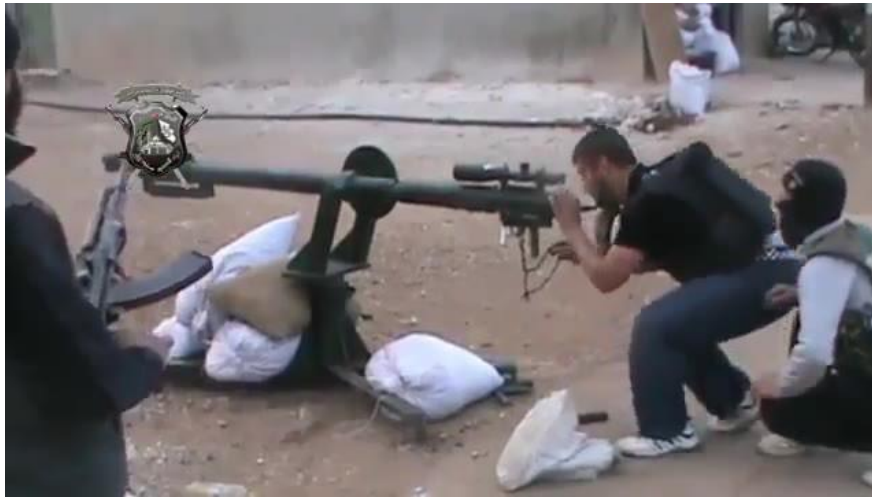
Fig. 14. Rifle manufactured based on 14.5 mm anti-aircraft gun's barrel Source: [Homemade 23 mm... n.d.].
