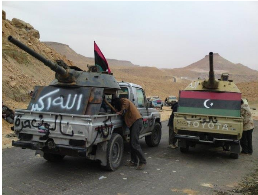
Fig. 7. Toyota vehicles with mounted BMP-1 turrets, Libya, 2013 Source: [Libyan technical... 2016].
