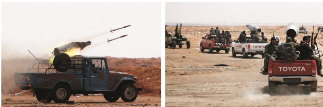
Fig. 8. Toyota vehicles with installed UB-32A-24 launcher-pod dismounted from Mi-24 helicopter Source: [Taylor 2011].
