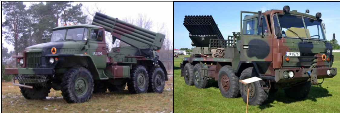
Fig. 3. On the left – 122 mm BM-21 rocket launcher, on the right – 122 mm RM-70/85 rocket launcher Source: [7].
