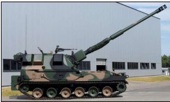
Fig. 1. 155 mm self-propelled howitzer Krab – first prototype on a chassis of the Korean K9 howitzer Source: [5]
