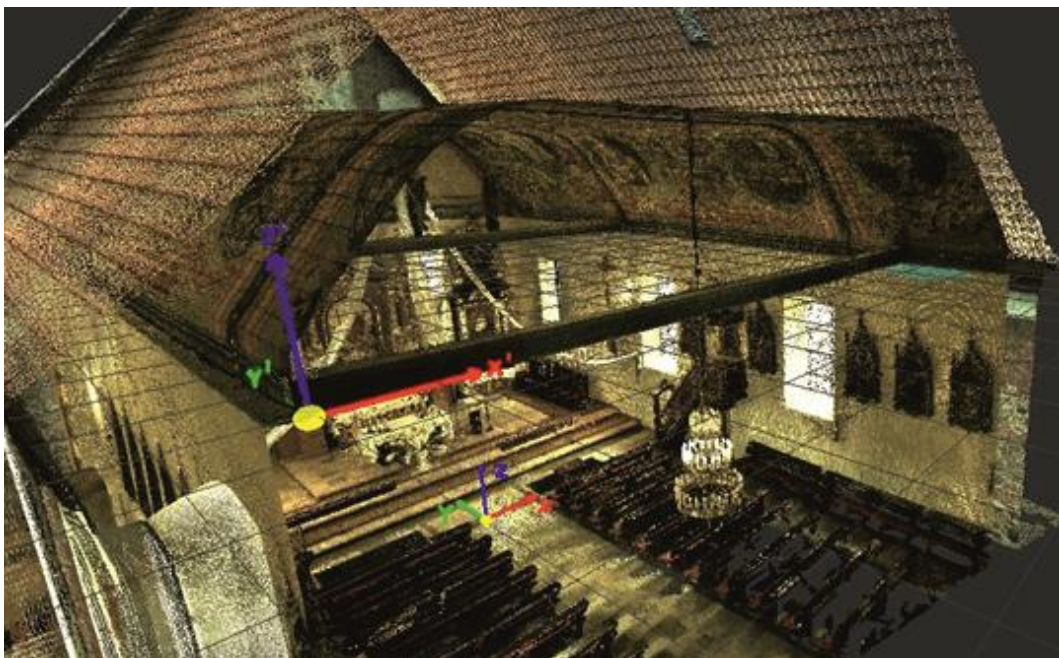
Fig. 6. Established coordinate systems: ( XYZ ) on the floor and ( X'Y'Z' ) on the beam Source: Own work.
