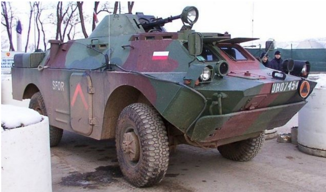
Fig. 4. BRDM-2M96 used by SFOR (Bosnia). The introduced modifications, including side doors and a spare wheel on a holder at the back of the hull, can be clearly seen Source: [12].
