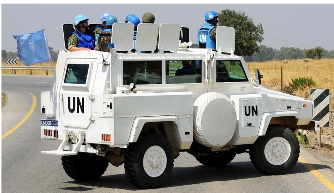
Fig. 2. Armoured personnel carrier RG-31 Nyala used during UNDOF mission. One can clearly see open top hatches with landing forces soldiers Source: [6].
