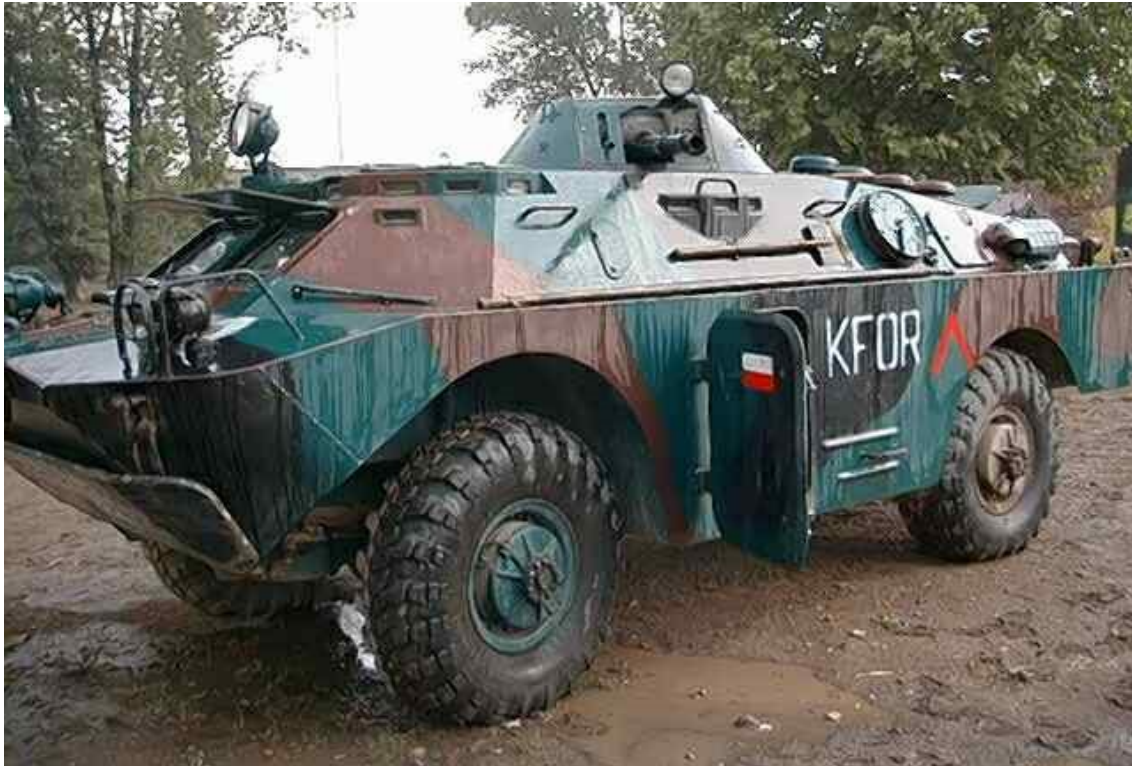
Fig. 7. BRDM-2M96 used by KFOR (Kosovo). An element attracting attention is the open side door Source: [18].
