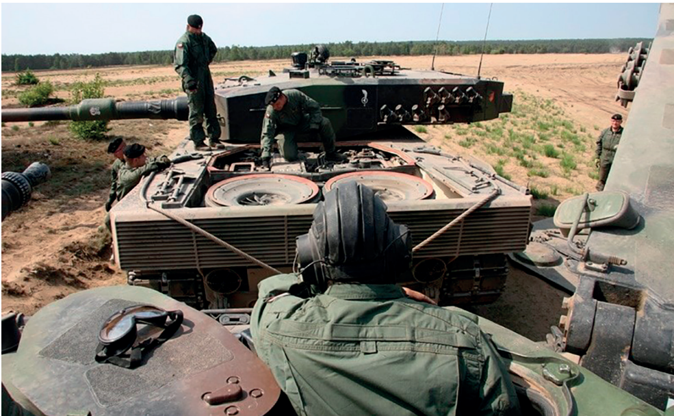
Fig. 3. The crew of a Leopard 2A4 and Bergerpanzer tank with 10BK Panc during the replacement of a MB 873 engine in training ground conditions.
