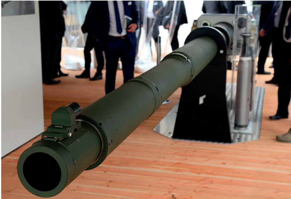
Fig. 1. The 130 mm tank gun demonstrator, developed for the tank of the new generation, is often referred to as “Leopard 3” Source: [10].
