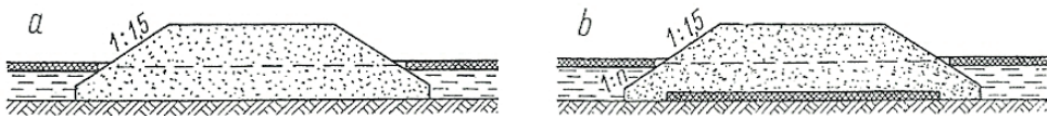
Fig. 4. Cross-sections of embankments founded on irrigated marshes: a – embankment on the mineral marsh bottom, after removing the peat carpet, b – embankment on a peat carpet lowered to the mineral mud bottom (under the weight of the embankment) Source: [5, 9].
