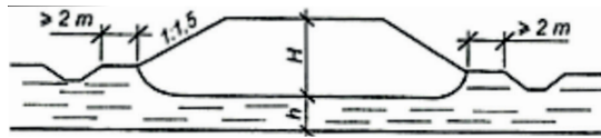
Fig. 3. Embankment which is partially submerged in peat deposits, after its partial removal. The solution is applied when crossing marshes filled with peat of solid consistency: H – height of the embankment with its part below ground level, h – thickness of peat layer, left under the bottom of the embankment Source: [9].
