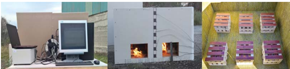
FIGURE 4. MEASUREMENT PANEL AND SMALL-SCALE DWELLING MODEL FOR THE MEASURING OF TEMPERATURE DEVELOPMENT OF THE SELECTED MATERIALS
