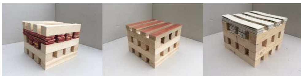
FIGURE 2. FUEL SOURCE – FUEL CRIBS
