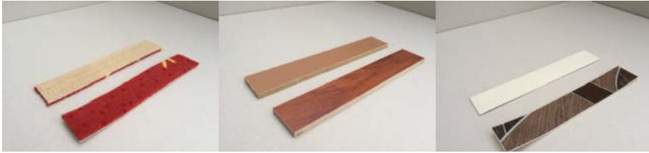
FIGURE 3. FUEL SOURCE. LEFT: POLYAMIDE, MIDDLE: LAMINATE, RIGHT: VINYL
