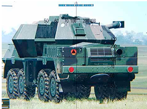
Fig. 2. 152 mm AHS DANA – view through fire officer's observation device Source: Own study (VBS image).
