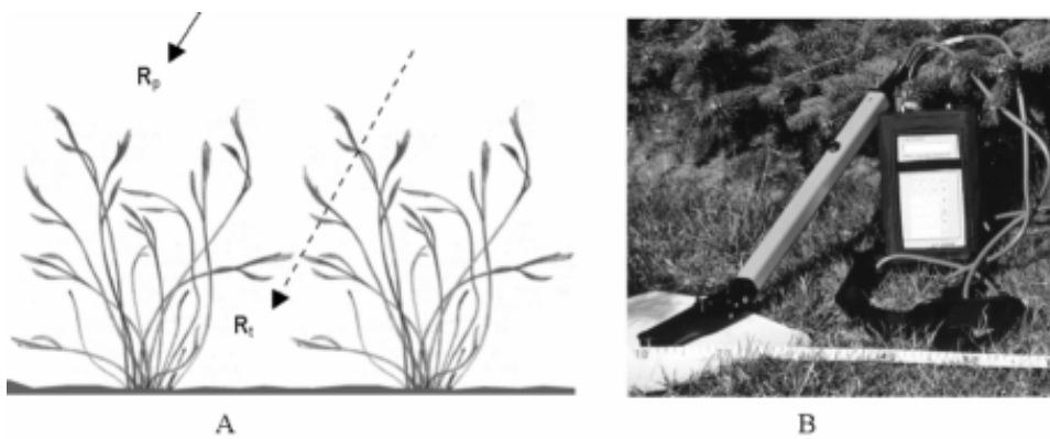
Fig. 8. A) Scheme of LAI measurements: measurement of sky brightness above the canopy and light transmitted measured below the canopy, B) LAI-2000 Plant Canopy Analyser.
