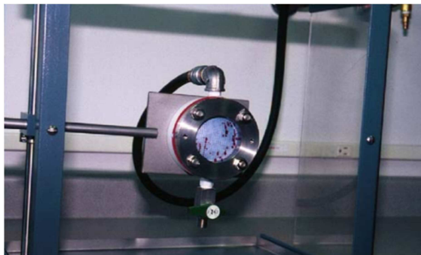
Fig. 9. The study of diffusion in the configuration used in the ATSM f903 [1]
