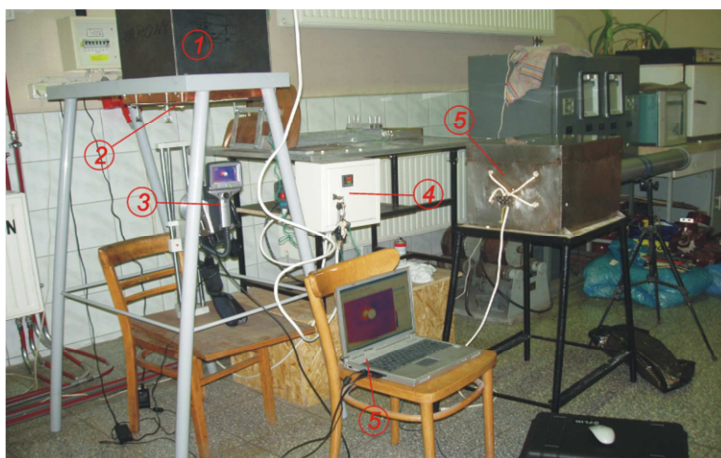
Fig. 16. The thermal measurement of the temperature of the sample irradiated by blackbody
