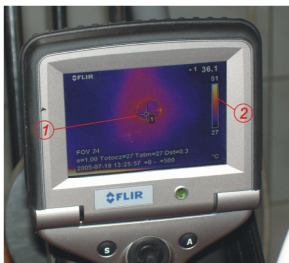
Fig. 17. The monitor of the thermal imager with a visible internal thermal image of the specimen
