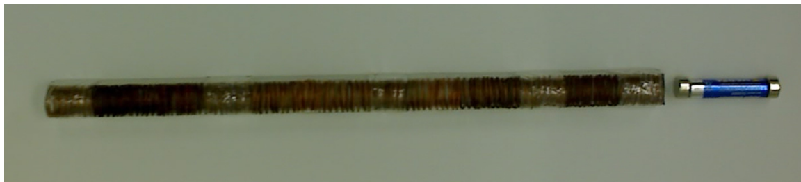
Photo 1. An example of the simplest, linear electric motor.
