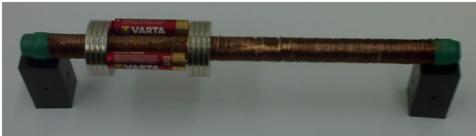
Photo 4. External appearance of one of the two linear electric motors with a cylindrical guide.
