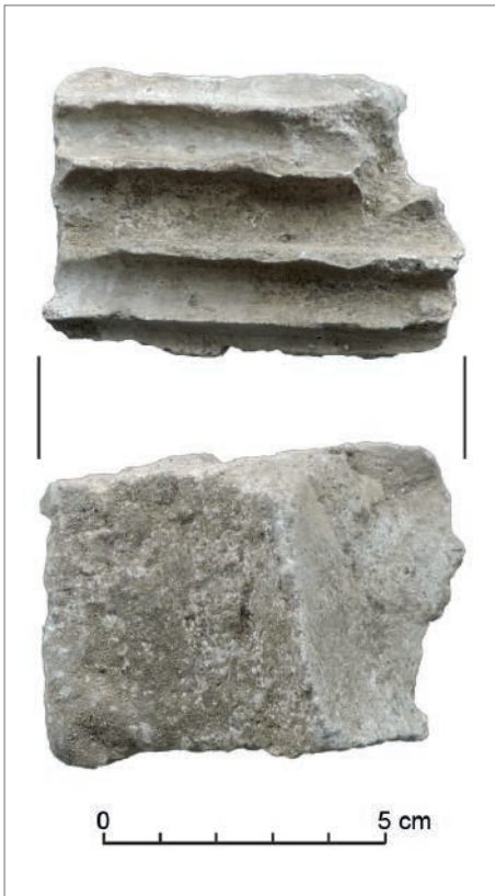
Fig. 12. Fragment of a lime-mortar ceiling with imprints of reed bunches and wooden beams (University of Warsaw Marea Archaeological Project | photos M. Gwiazda)
