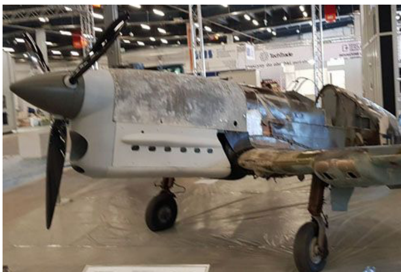
Figure 5. French fighter plane Caudron CR-714 Cyclone with added parts made by large format 3D printing technology: full cover engine, front the radiator and three-blade propeller spinner(Photo: Jakub Link-Lenczowski via [8])
