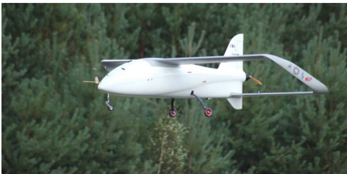
Figure 7. Dynamically similar flying model of an aircraft in the MOSUPS aircraft in the system of interconnected wings made by the MSP company within the research project of the Institute of Aviation, ITWL, Warsaw University of Technology and MSP [15]
