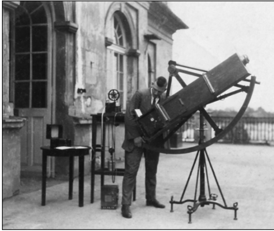
Fig. 11. Chronocinematograph – a tool to obtain a special film during a solar eclipse. Kazimierz Kordylewski on the terrace of the Astronomical Observatory in Kraków, 1926 (The Jerzy M. Kreiner private collection)
