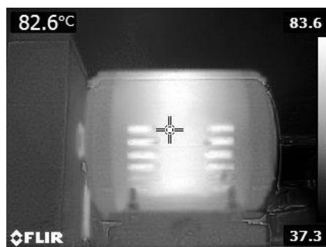
Figure 1. Thermographic picture of a motor reaching 82.6 C°.
