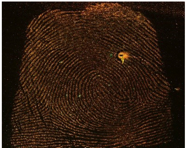
Fig. 33. Fingerprint revealed on a ceramic plate using the NANODAK 40 suspension, registered in UV light of the wavelength of 360 nm, with a yellow filter
