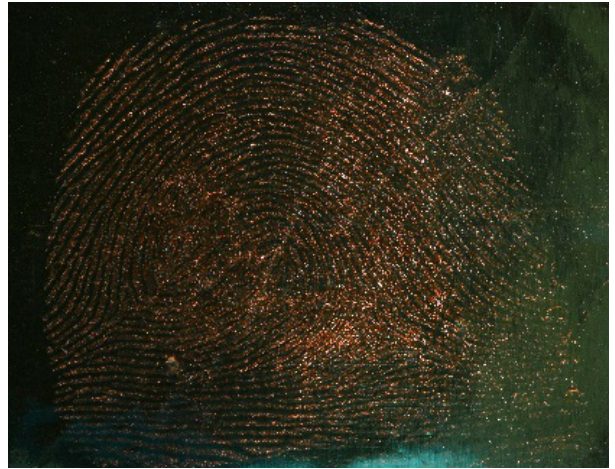
Fig. 38. Fingerprint revealed on an aluminium foil using the NANODAK 40 suspension, registered in UV light of the wavelength of 360 nm, with a yellow filter
