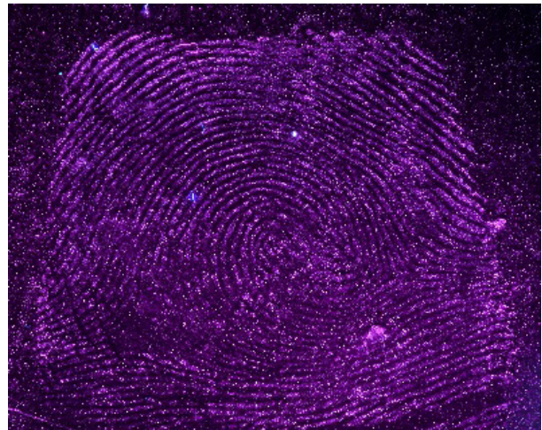
Fig. 22. Fingerprint revealed on a ceramic plate using the NANODAK 30 suspension, registered in UV light of the wavelength of 360 nm, with a colourless filter
