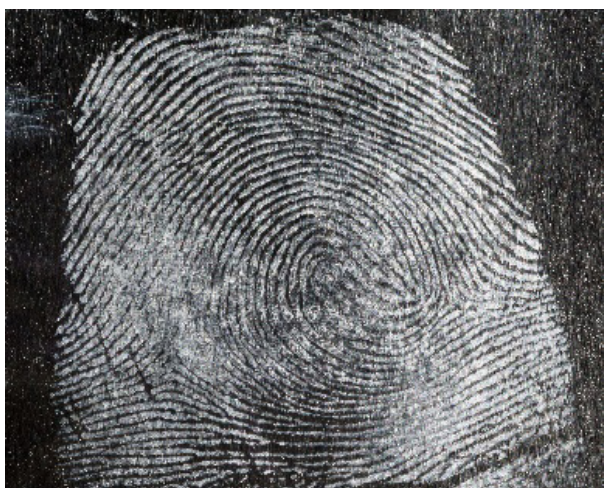
Fig. 42. Fingerprint revealed on an aluminium foil using the NANODAK 1 nanopowder, registered in white light
