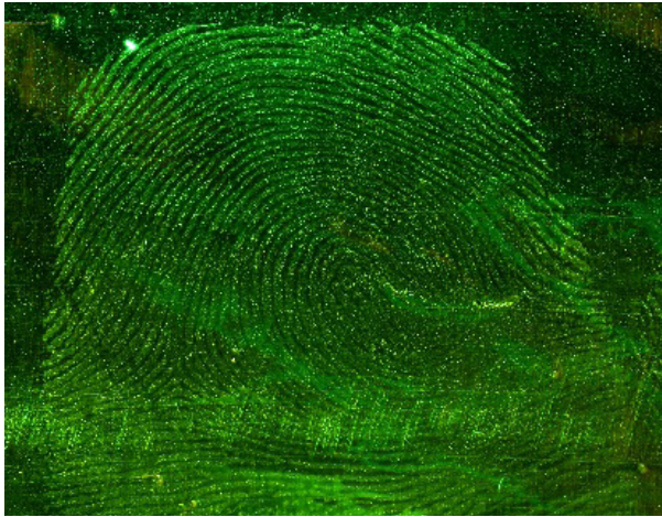
Fig. 29. Fingerprint revealed on an aluminium foil using the NANODAK 30 suspension, registered in blue light of the wavelength of 410 nm, with a yellow filter
