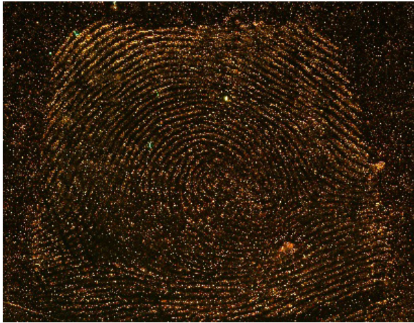
Fig. 23. Fingerprint revealed on a ceramic plate using the NANODAK 30 suspension, registered in UV light of the wavelength of 360 nm, with a yellow filter
