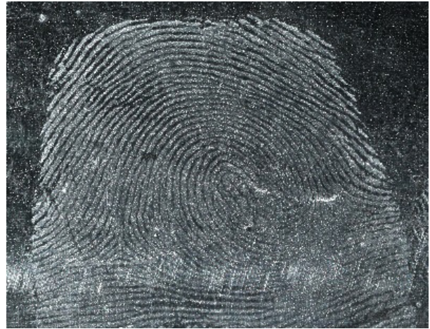
Fig. 26. Fingerprint revealed on an aluminium foil using the NANODAK 30 suspension, registered in white light
