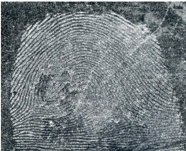
Fig. 36. Fingerprint revealed on an aluminium foil using the NANODAK 40 suspension, registered in white light
