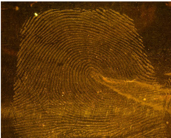
Fig. 30. Fingerprint revealed on a ceramic plate using the NANODAK 30 suspension, registered in blue light of the wavelength of 410 nm, with an orange filter
