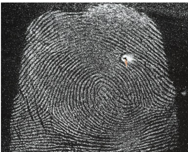
Fig. 31. Fingerprint revealed on a ceramic plate using the NANODAK 40 suspension, registered in white light
