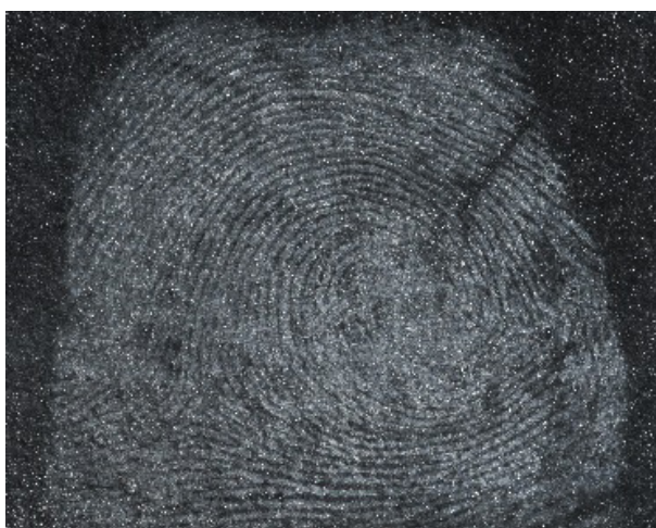
Fig. 43. Fingerprint revealed on a cardboard folder using the NANODAK 1 nanopowder, registered in white light
