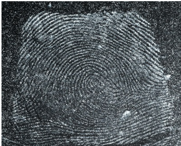
Fig. 21. Fingerprint revealed on a ceramic plate using the NANODAK 30 suspension, registered in white light
