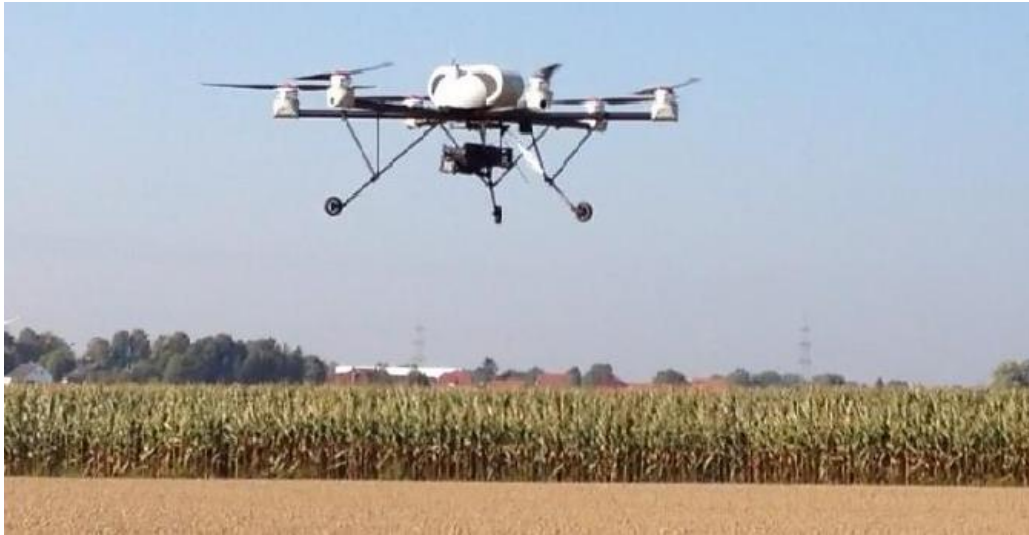
Fig. 10. A drone with a lidar contamination detector
