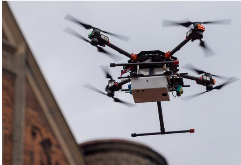
Fig. 8. Unmanned Aerial Vehicle - AGH for air pollution control; tests in Bytom; laser dust concentration meters, CO and CO 2 sensors used [13]
