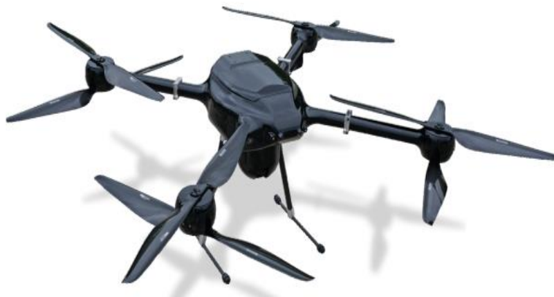
Fig. 7. Unmanned Aerial Vehicle (mini-UAV) – ATRAX take-off mass: 7÷22 kg; lift capacity: 15 kg; operating radius: 5 km; straight-line flight: <35 km; flight ceiling: <1000 m; flight time : 45÷60 min [12]
