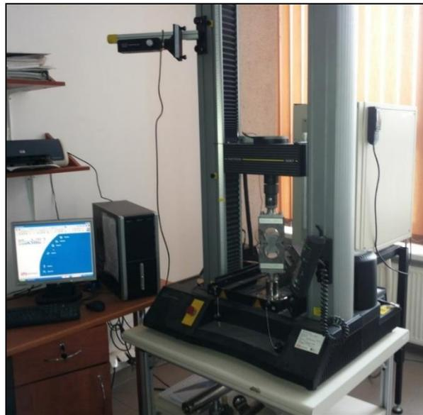
**Fig. 7.** The bench for testing the tensile strength
