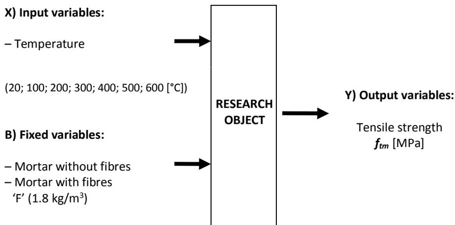
**Fig. 1.** The research program for determining the tensile strength  $f_{tp}$
