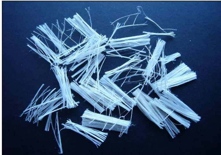
**Fig. 2.** The polypropylene fibers Fortatech® Fibre High Grade
