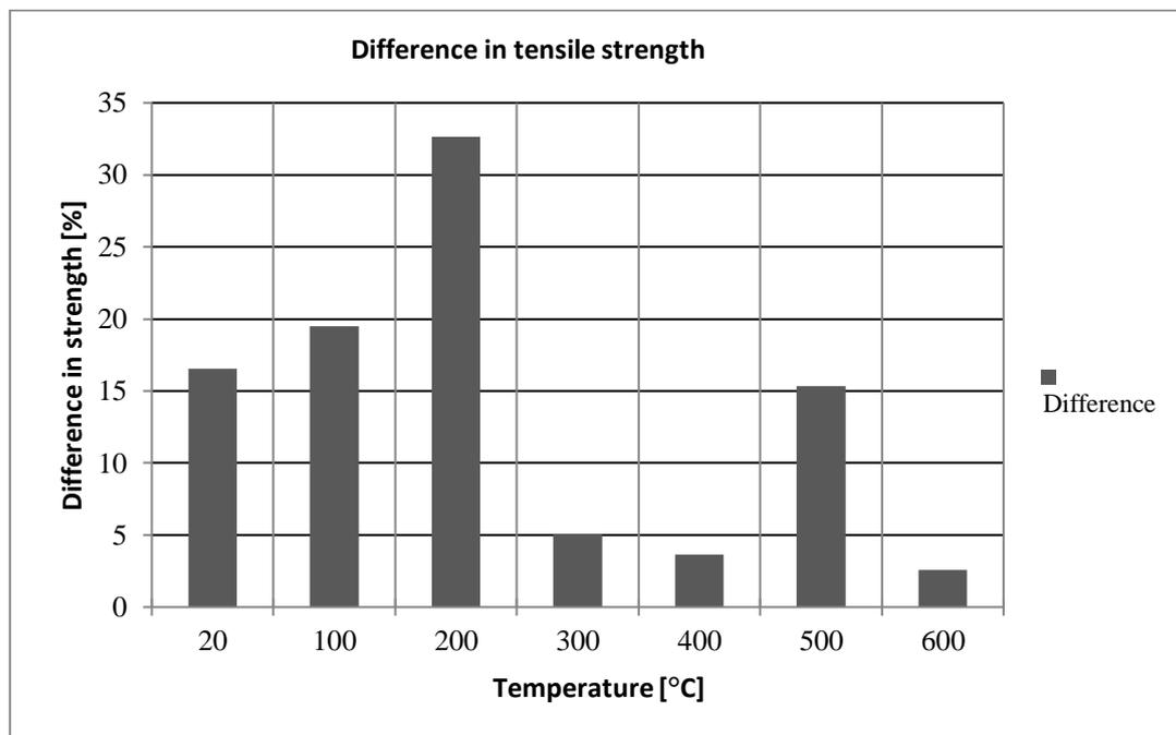
**Fig. 10.** Differences in strength between samples without and with the addition of polypropylene fibers
