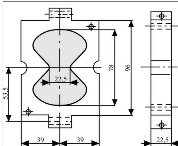
**Fig. 3.** The steel mold for the preparation of octal specimens for testing
