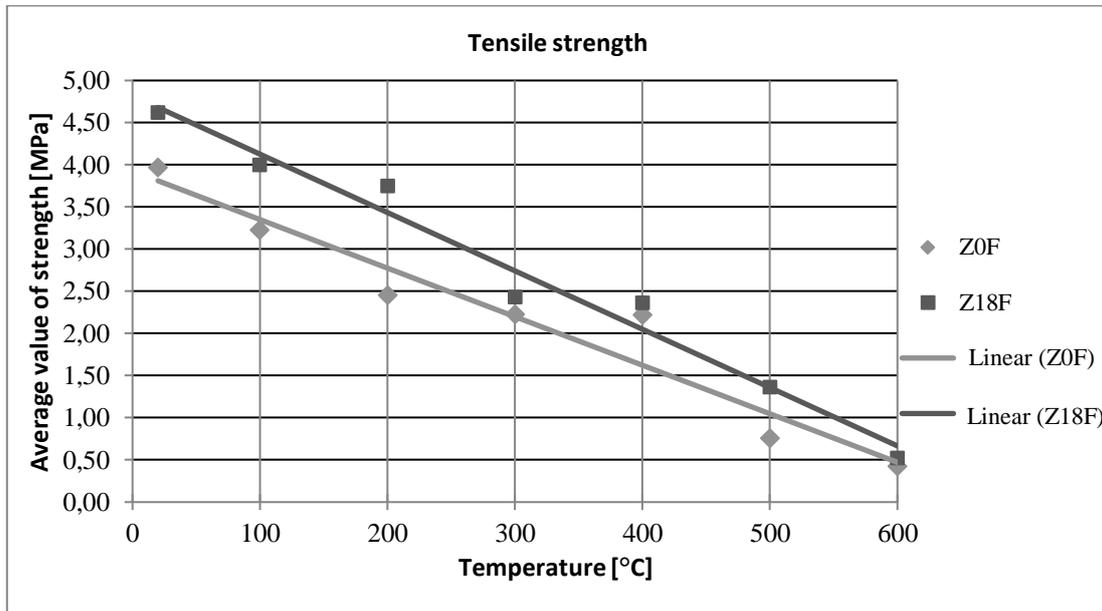
**Fig. 9.** The summary of average tensile strengths of mortar samples without and with the addition of polypropylene fibers at various temperatures (a graph with the trend line)
