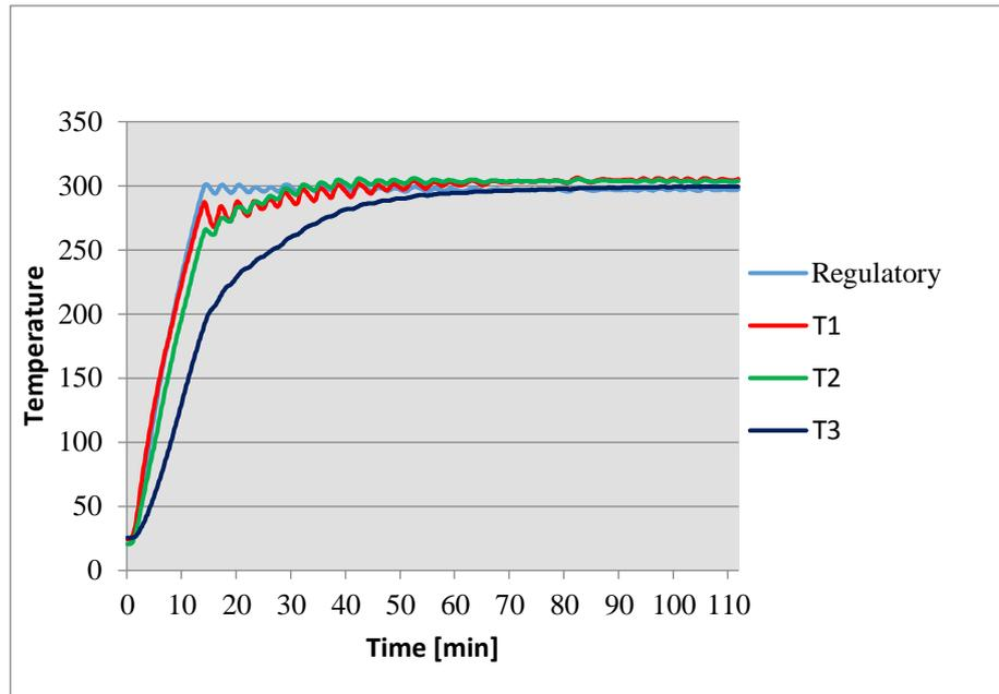
**Fig. 6.** The heat-soaking process – the temperature of 300°C
