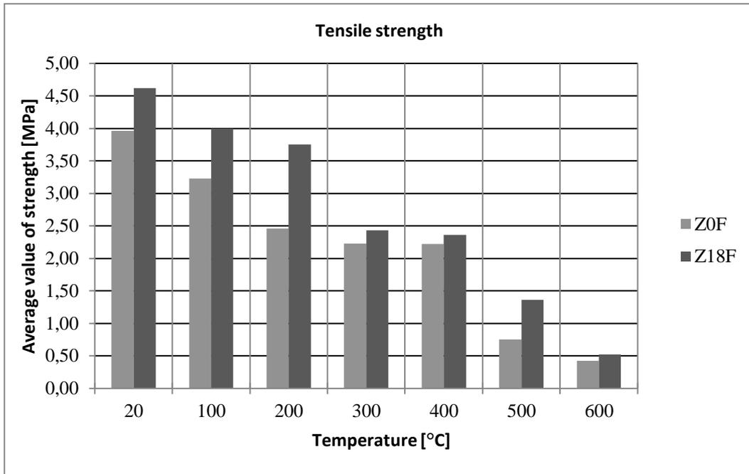
**Fig. 8.** The summary of average tensile strengths of concrete samples without and with the addition of polypropylene fibers at different temperatures
