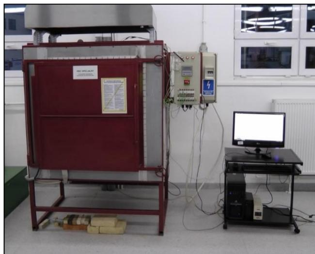
**Fig. 4.** The bench for heating the samples
