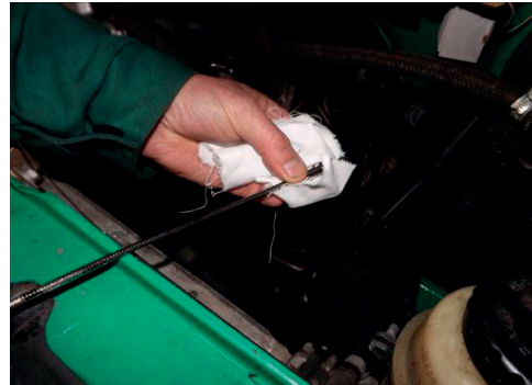
Fig. 6. Checking the oil level in the engine Source: Own materials.
