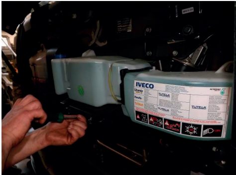
Fig. 5. Checking the filter cleanliness Source: Own materials.
