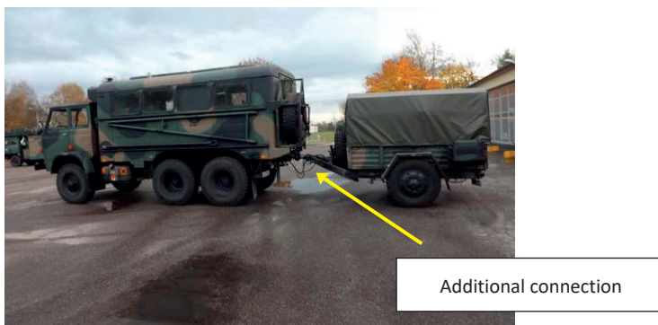
Fig. 7. Example of connecting a car with a trailer – securing with an additional connection Source: Own study.
