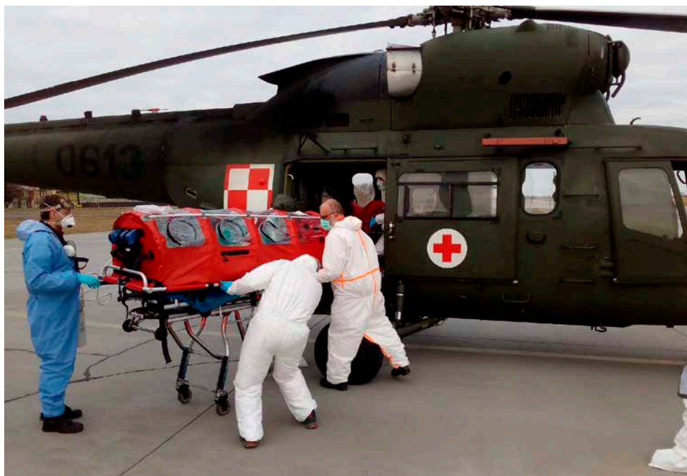
Fig. 1. Placing a patient inside the W-3 military helicopter using the Bio-Bag isolation chamber Source: [7].
