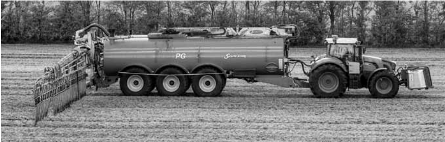
Figure 6 Complete set driving on the field for providing spreading of acidification slurry
