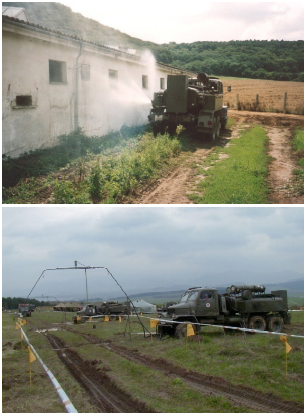
FIG. 3 CHEMICAL PV3S THE SPRAY TRUCK/ADR – 12 M IN THE DECONTAMINATION OF GROUND
