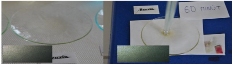
FIGURE 4 GASOLINE SAMPLE BEFORE THE EXPERIMENT, AND WITH \text{HNO}_3 IN A RATIO OF 1:1 AT 60 MINUTES AND MICROSCOPIC IMAGES
