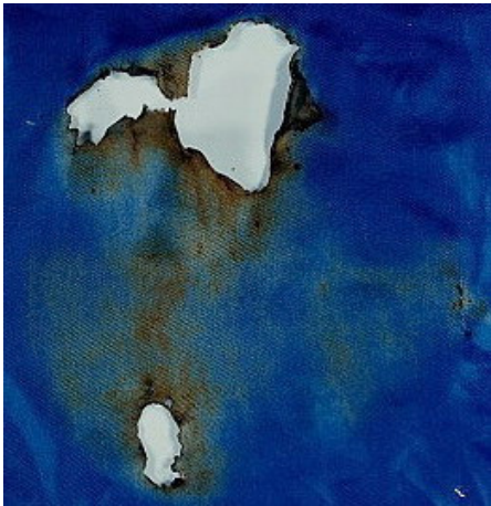
FIG. 2. THE PIECE OF FABRIC DAMAGED UNDER THE ACTION OF HIGH TEMPERATURE.
