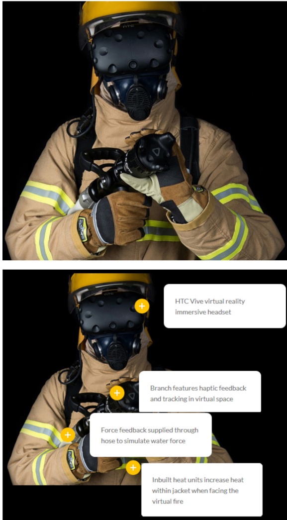
FIG. 1. FLAIM TRAINER™ PLACES FIREFIGHTERS IN THE REALISTIC TRAINING SCENARIO AVAILABLE BY UTILISING SEVERAL CUSTOMISED ELEMENTS.
